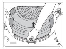
3. Open the filter pressing the button, among two slots on fingers. Clean the filter using dump hand or cloth. After a period of time, a patina due to detergent residue on laundry forms on the filters. When this occurs, clean the filter with warm water using a brush.
